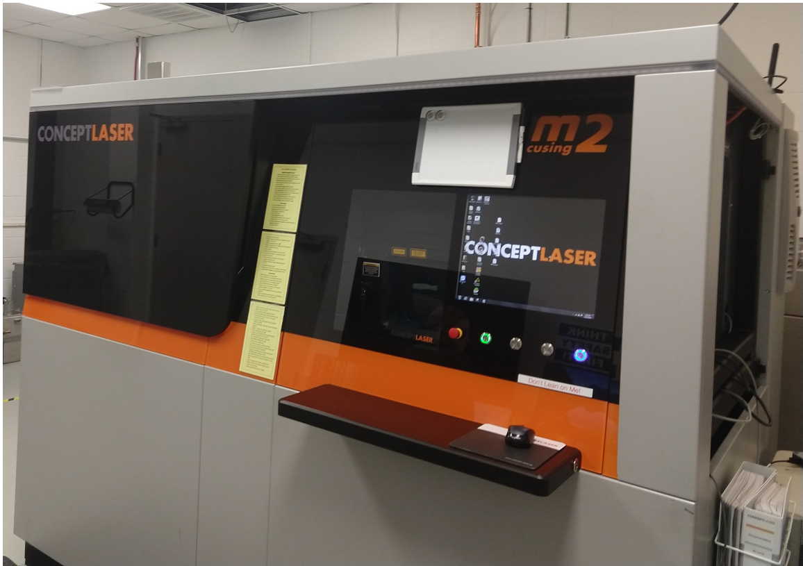
Figure 11. ConceptLaser Cusing M2 3D Printer used to produce test components.
